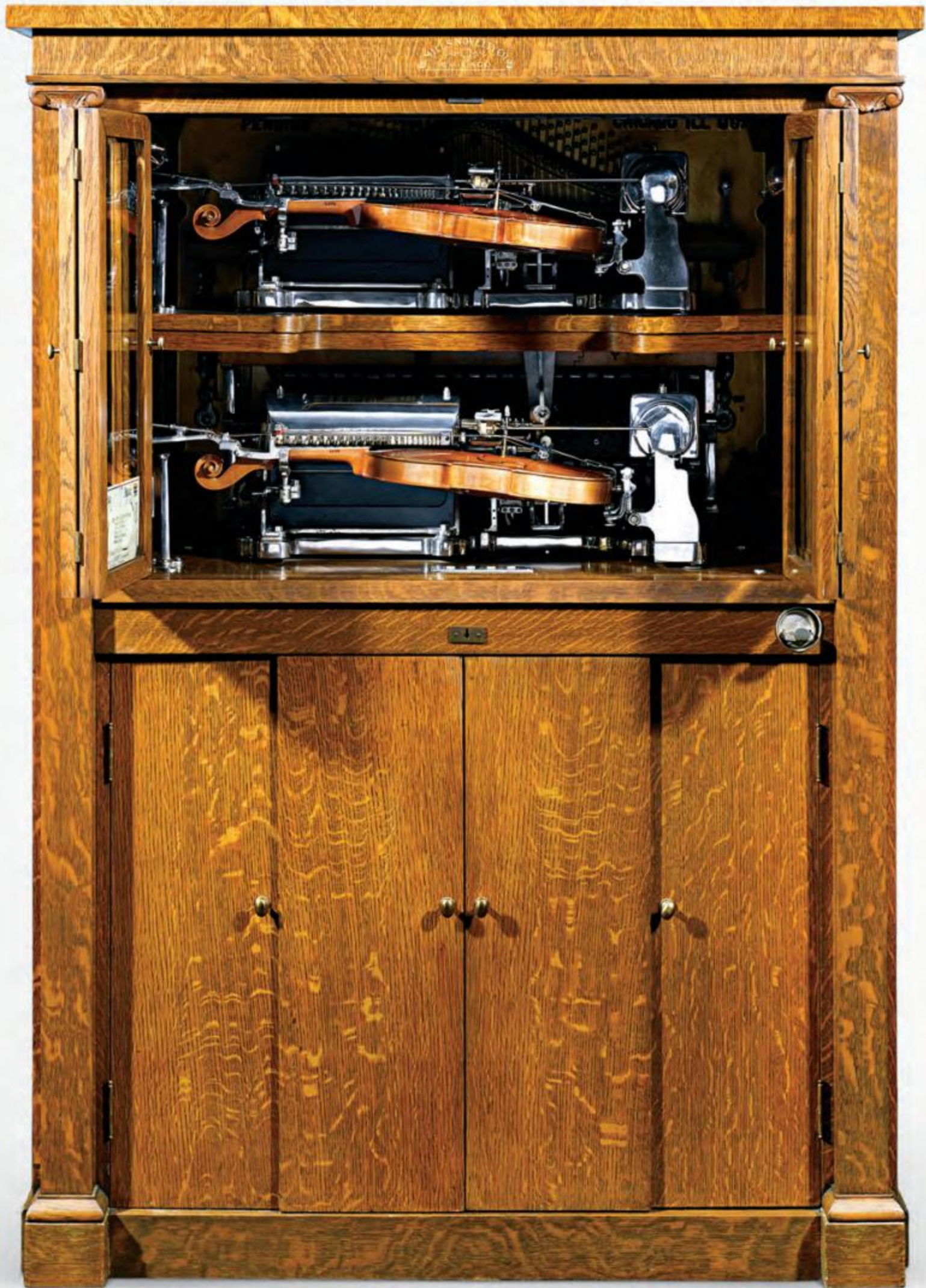
The Double DeLuxe model contains two independently playing four-string violins with the ability to reproduce 64 notes, as well as a 44-note piano.
